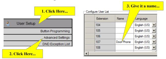
Do this instead: This example is using Extension 107 (Analog Station Port) for the Door Phone.
