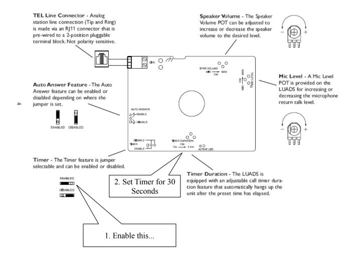
Since there is no Disconnect Signal from the Analog Station Ports on the Combo Card, you need to have the Door Phone disconnect itself automatically after a period of time.
