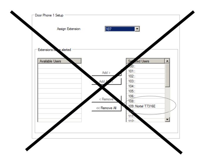
Instead of using the Door Phone function, we will put a Calling Group (74) number as a Hot Line Alert Number in the extension that is used as a Door Phone.
